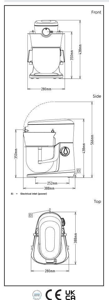
Electric Supply voltage: 602201 (EMX5\_PRO) 200-240 V/1N ph/50/60 Hz **Total Watts:** 0.5 kW Capacity: Performance (up to): 0.75 kg/Cycle
